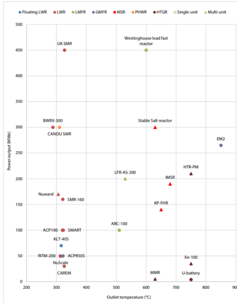
Figure 1: Selected reactor designs as a function of power output, core outlet temperature and deployment configuration
